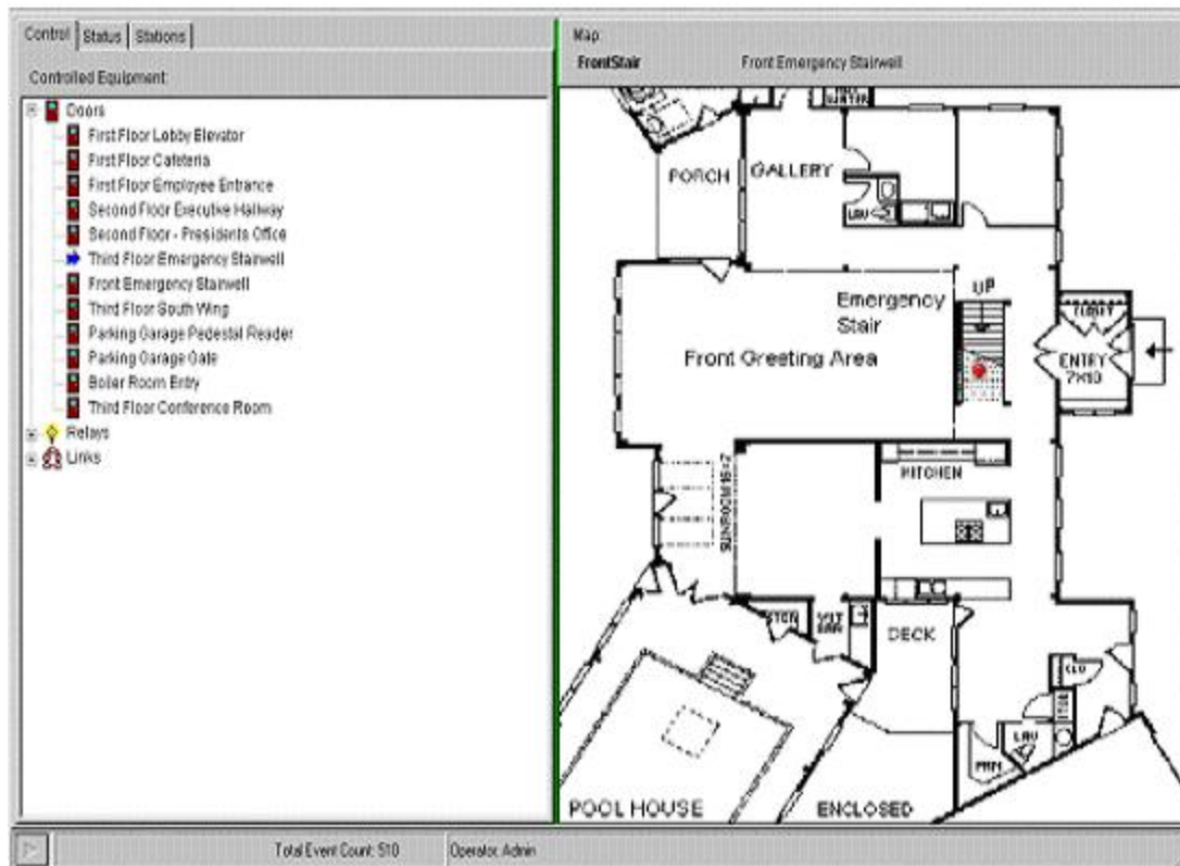
Fig. 3.7. Map area on the right showing bitmap of Third Floor Emergency Stairwell device highlighted on the left.
